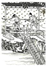
One of the inventions that allowed the Chinese to make use of water was the square-pallet chain pump. It consists of an endless circulating chain bearing square pallets, which hold water, soil or sand. No specific records of origin exist but accounts of the philosopher Wang Ch'ung in 80 CE describe it. This pump can haul enormous quantities of water from lower to higher levels. A single good pump can lift water 15 feet. By medieval times in China the pumps
